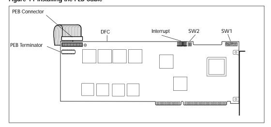
5. Insert the DVCs and connect the PEB cable to each card.
